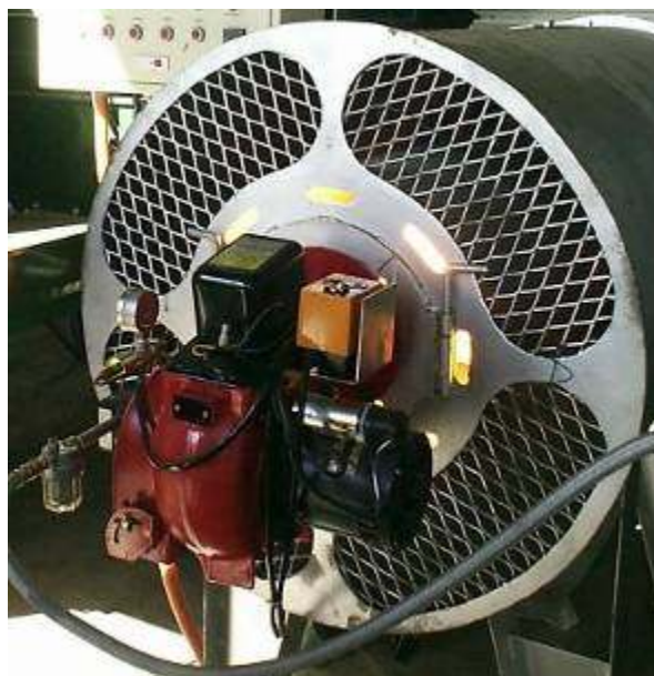
Figure 28: Kerosene burner attached at air heater of a re-circulating batch dryer
