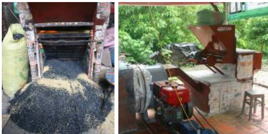
Figure 29: A simple Vietnamese inclined grate rice hull furnace for a flat bed dryer with 6-8 t capacity (left) and the improved NLU-Hohenheim-IRRI semi-automatic, down-draft furnace for more even burning, cleaner combustion and lower labor requirement (right)
