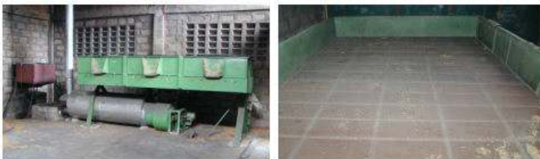
Figure 15: Kerosene fired tilted-bed dryer for easy unloading (left), drying bin with perforated false floor (right)
