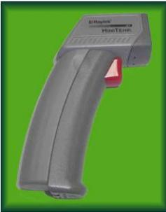
This non-contact thermometer can be used for monitoring grain temperature in post harvest processes like rice milling and drying.
