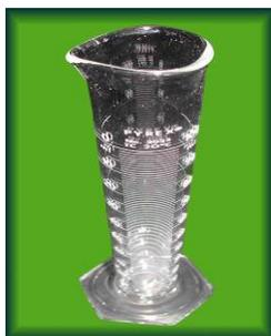
This cylinder for volumetric measurements is calibrated and is easy-to-read. Raised graduation allows precise measuring of the volume of grain samples.
