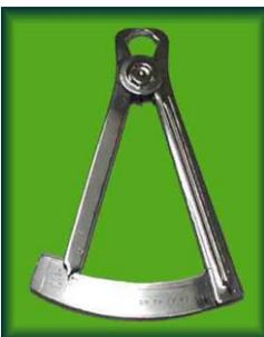
The caliper can be used to measure the length and width of the grain
