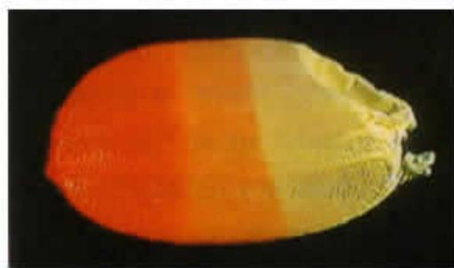
Cracks in grain as seen through a red light filter
