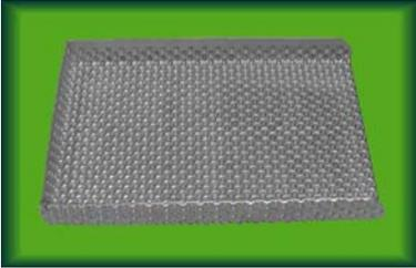
These trays are used to separate the broken rice (large and small) from the whole kernel. By oscillating the trays, broken rice remains in the indents while the head rice falls off the grader.
