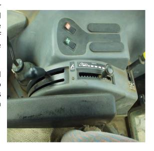
**Drop valve** This controls the speed of drop of the implement attached to the tractor. Excessive speed of the drop may cause damage or injury. Adjust the speed of drop slow enough for safe operation.
