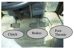
**Clutch pedal.** The clutch is used to disengage the drive train from the engine and change gears. It is always good practice to depress the clutch before starting and stopping the engine. The clutch is also used to engage or disengage the power-take-off drive.
