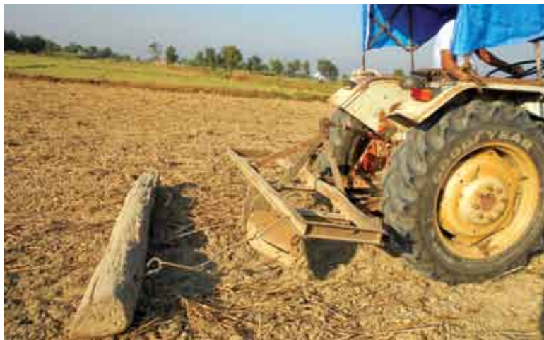
Land leveling using a scraper (Raiser) and planking
